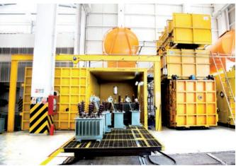
After drying the transformers whose assembly of active part is completed, in the drying furnaces at 120 degrees Celcius are put into tanks and filled with oil in the vacuum chamber. The air entrapped in the transformer tank is removed by the suction effect in the
